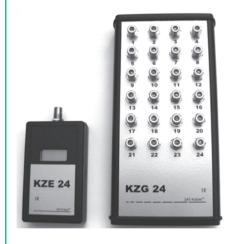
This device is designed for assignment of coaxial cables (antenna cables) of a in-house installation to the corresponding system outlets and reverse. The assignment is also possible over star- and treedistribution systems. It consists of a basic device KZG 24 (line transmitter for 24 lines) and an evaluation device KZE 24 (receiver). By an appropriate coupling it is possible to carry out the check up under normal operating conditions of the network.
