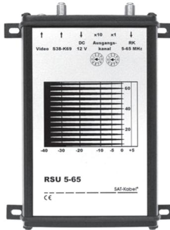
The Return path spectrum converter (analyser) *RSU 5-65* scans the signals of the return path (5-65 MHz) and convert this graphic representation in a free selectable TV-channel in the range of S38-Ch 69. Thus the return path signals of the CATV system under test can be displayed with an usual TV set.
